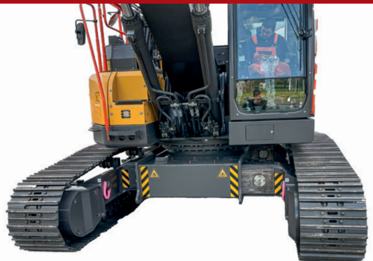
Telescopic tracked undercarriage
